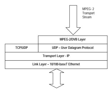
Figure 3.8: IP Output Protocol Stack
